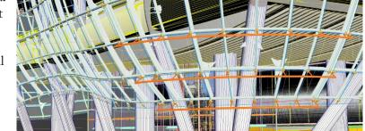
Figure 5: Typical View of Awning Protection Bars (Shown in orange color) Rendering courtesy of TJPA
