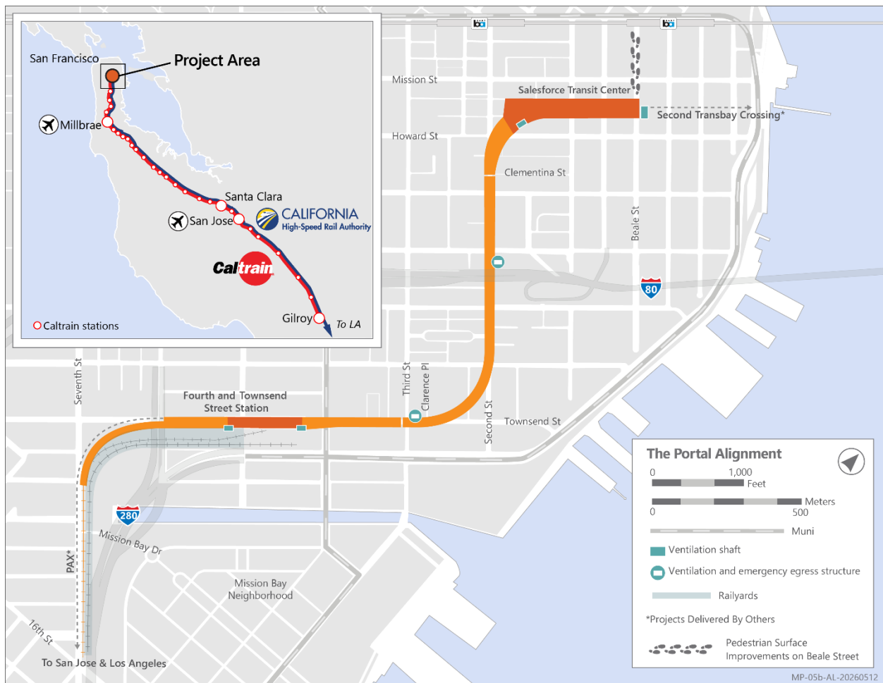
Figure 1. The Portal Alignment and Major Components
