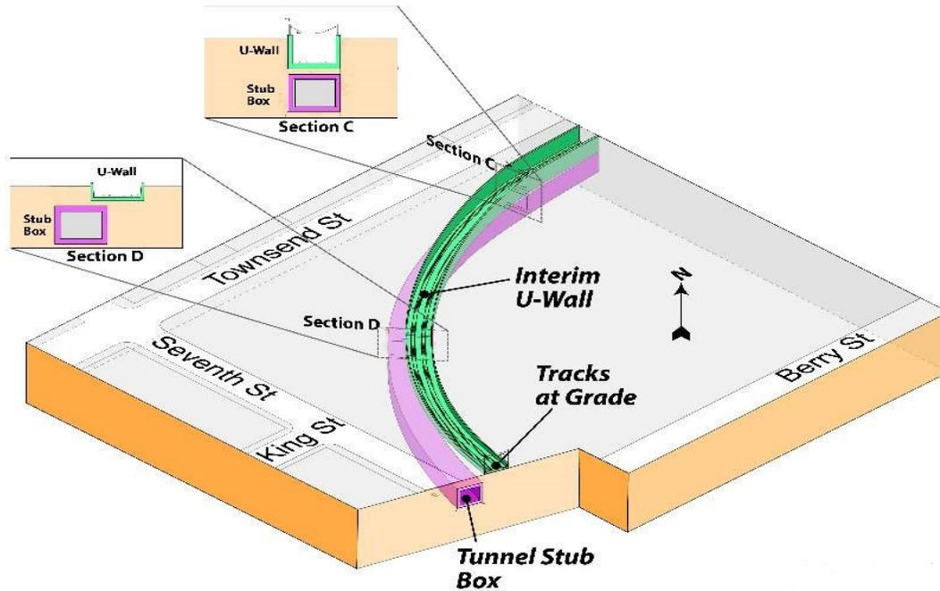
**Figure 11. 2018 Tunnel Stub Box at Caltrain Railyard**
