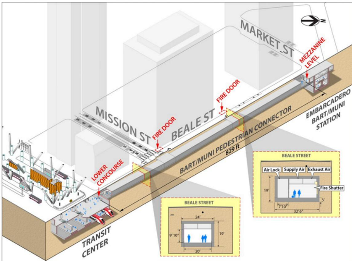
**Figure 2. BART/Muni Pedestrian Connector to be Deferred**
