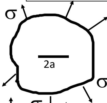
Arbitrary crack in a plate subjected to  $\sigma$
