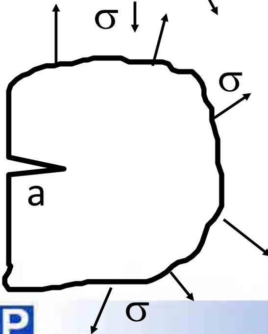
Fracture occurs when the applied stress intensity ( $K$ ) exceeds the fracture toughness ( $K_{1c}$ ) of the plate material
