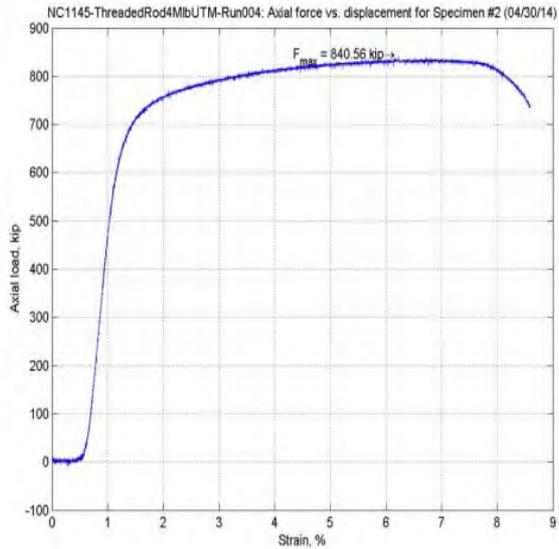
Strain testing to design limits
