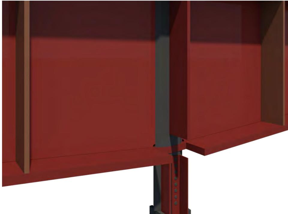
Grind the flame-cut surface of the web hangers to a smooth surface, and Magnetic Particle test.
