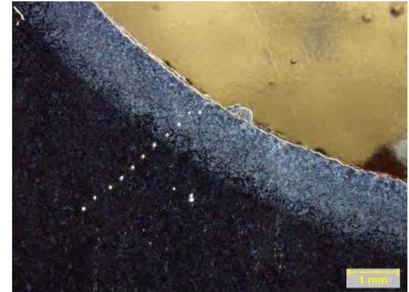
Vickers Microhardness measurement Locations, Specimen Center.
