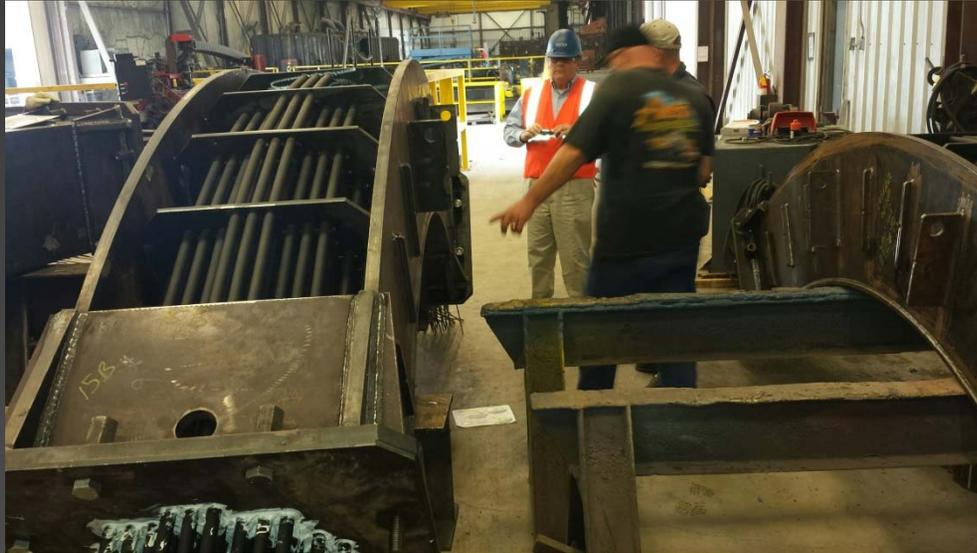
Above and Right: Quality Control and Assurance visit to VSL in Fort Worth, Texas. Observed fabrication of cable saddles for the cable stay bridge. The bridge has a total of seven saddles.
