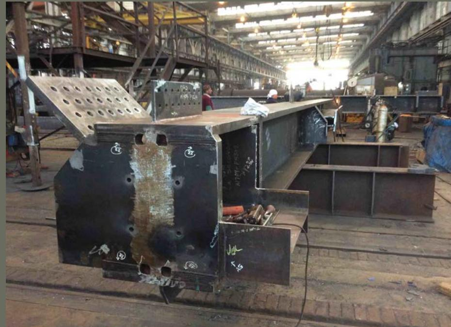
Tapered Beam in fabrication at Herrick shop in Southern California and Column (Lower Concourse to Transfer Girder) in fabrication at XKT shop in Vallejo.
