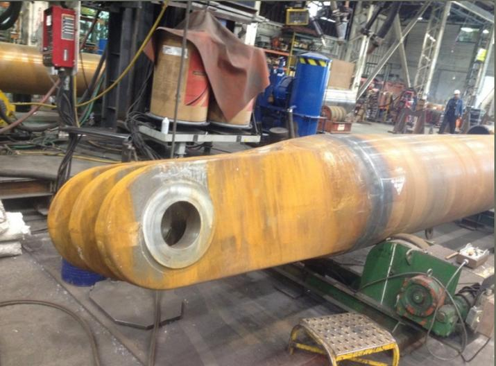
Work Proceeding at Oregon Ironworks – robot welding, cast node with attachment plates, cast node attached to pipe column.
