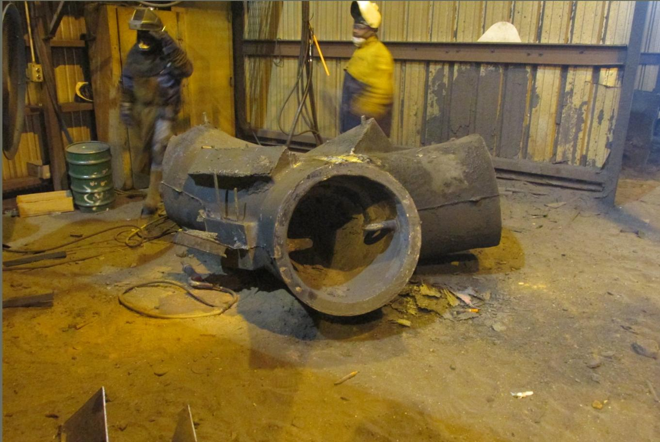
Type 21 Cast Node in Bradken's Amite, LA foundry, in "rough casting" form, prior to cleaning and shot blast.
