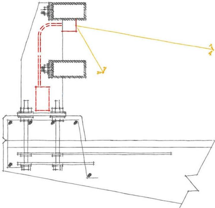
Section Through LED Light at Guardrail
