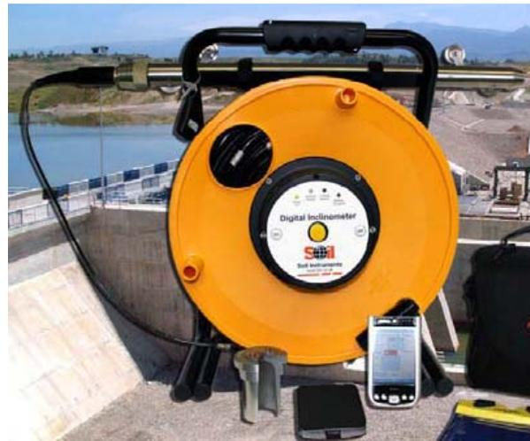
**Inclinometer and logging device**
