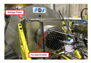
Figure 2-2 Cable East Anchor Head (Fixed)
