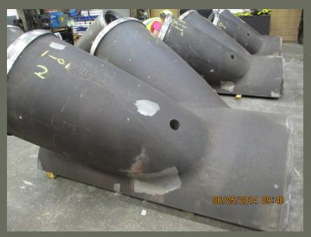
Node Type 1, machining completed, ready for inspection and shipping.
