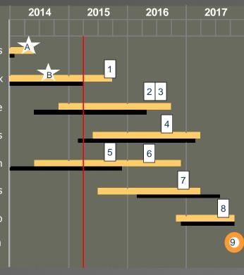
\* The current critical path of the project is as follows; structural steel fabrication and erection, eastern zone wall lift 2, lower concourse slab, wall lift 3 and rebracing.
