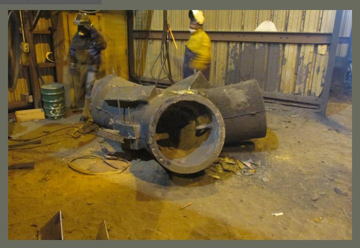
Type 21 Cast Node in Bradken's Amite, LA foundry, in "rough casting" form, prior to cleaning and shot blast.
