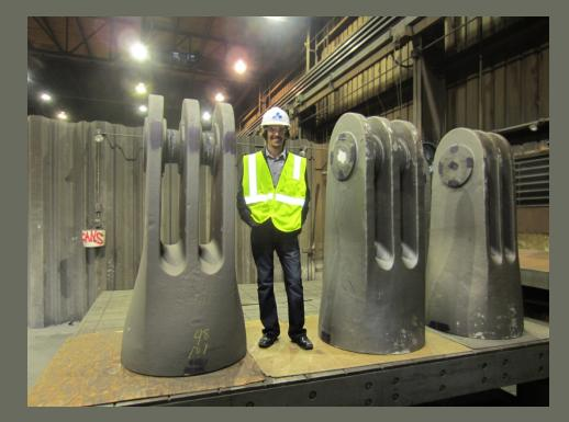
Type 71 and 72 Cast Nodes in Bradken's Kansas Foundry, preliminary cleaning and shot blast complete.
